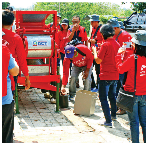
The operation of the PhilMech soybean sorter/ cleaner was demonstrated during training course held in Isabela.
