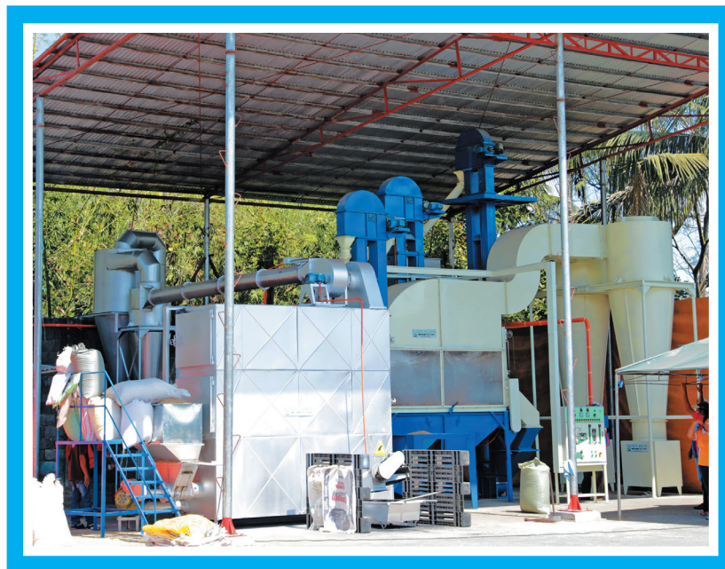
The pilot unit of the fluidized-bed dryer installed in Solano, Nueva Vizcaya for field testing.
